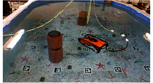
Fig. 2: Experimental setup: The 4 DoFs Seabotix LBV inside of the NTUA, Control Systems Lab test tank including obstacles.
