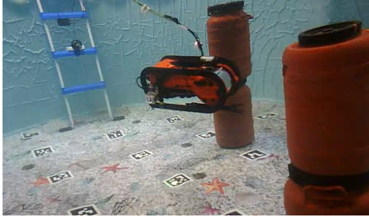
FIGURE 3.1: Experimental setup and problem formulation: the purpose of the controller is to guide the vehicle towards desired way points inside a constrained workspace including sparse obstacles.
