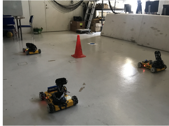
Fig. 1: The experimental setup demonstrating the proposed framework. Three Nexus 10011 mobile robots, in the workspace of Smart Mobility Lab (SML) [18] that contains 5 RoI.
